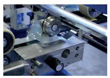
Electromechanical length measuring device:
